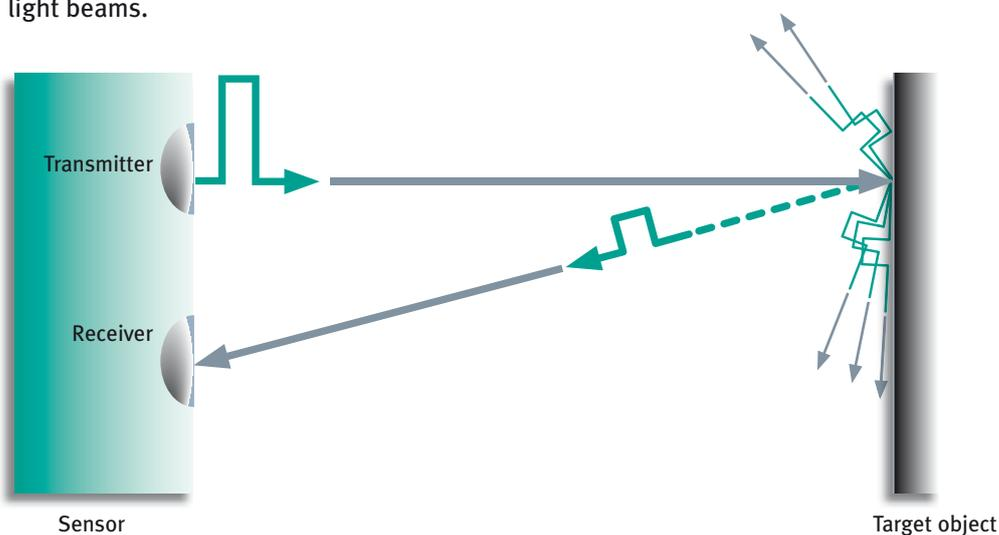
The times when the pulse was sent and received are measured extremely accurately.
