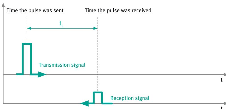
The exact distance ( $s$ ) from the object is calculated using the measured values ( $t_L$ ) and the speed of light ( $c$ ).
